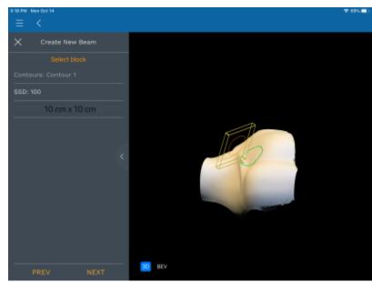
28. The user may then adjust any angles that need to be adjusted as well as fill in any free form text that needs to be sent to the Record and Verify (R&V) system. When the user is satisfied they may select *Save* and proceed to name the beam or leave the name at the default
