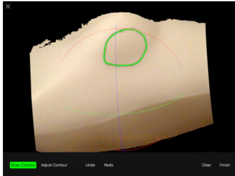
21. Once the user has completed the digitizing they may adjust the contour by selecting *Adjust Contour*. To do this the user needs to place the Apple Pencil or finger close to the area that needs to be adjusted and slide it to where it should be
