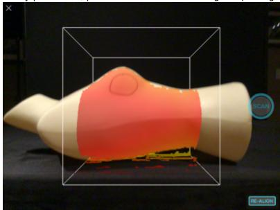
6. While the scan is active, the area that has been fully captured will appear white. You should continue scanning until the entire desired area is shown in white. For relatively smooth or flat areas, the scan can be obtained within 1-2 seconds without moving the iPad, but for larger or highly curved areas, you may need to slowly move or rotate the iPad to capture the entire patient surface.
