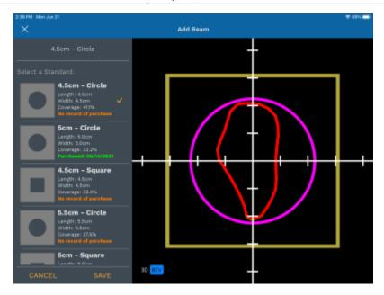
When a standard block is selected for a beam the original patient contour will be displayed along with the standard block shape. The selected standard block shape will then be used for ordering and DICOM export of that beam/block.
