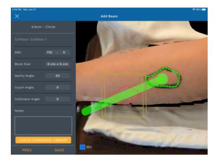
The top 10 best fitting supported standard blocks for the current cone size that are larger than the contour will be displayed to the user based on a coverage ratio (digitized area / block area). If applicable, at least two of the top fitting standard blocks will include any previously purchased standard blocks.
