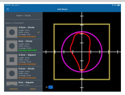
Users may select a standard block from the list, causing the original patient contour to be displayed along with the standard block shape, allowing users to make a visual assessment of the quality of fit for each standard block. If saved, the selected standard block shape will be stored to the beam and then be used for ordering and DICOM export of that beam/block. Ordering a standard block will automatically add it to the user's purchase history as well.
