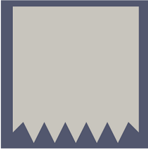
Fig. 5: Aperture no mill radius or smoothing
