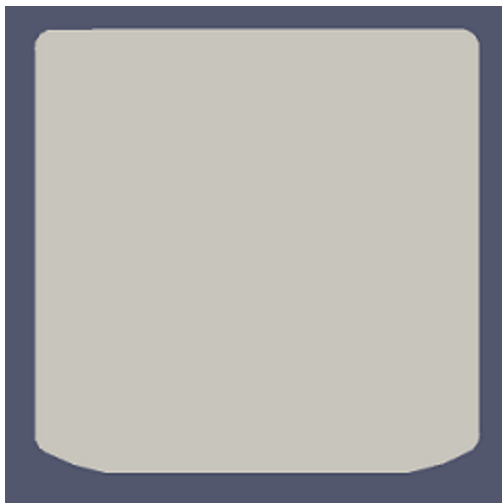
Fig. 7: Aperture with mill radius and smoothing
