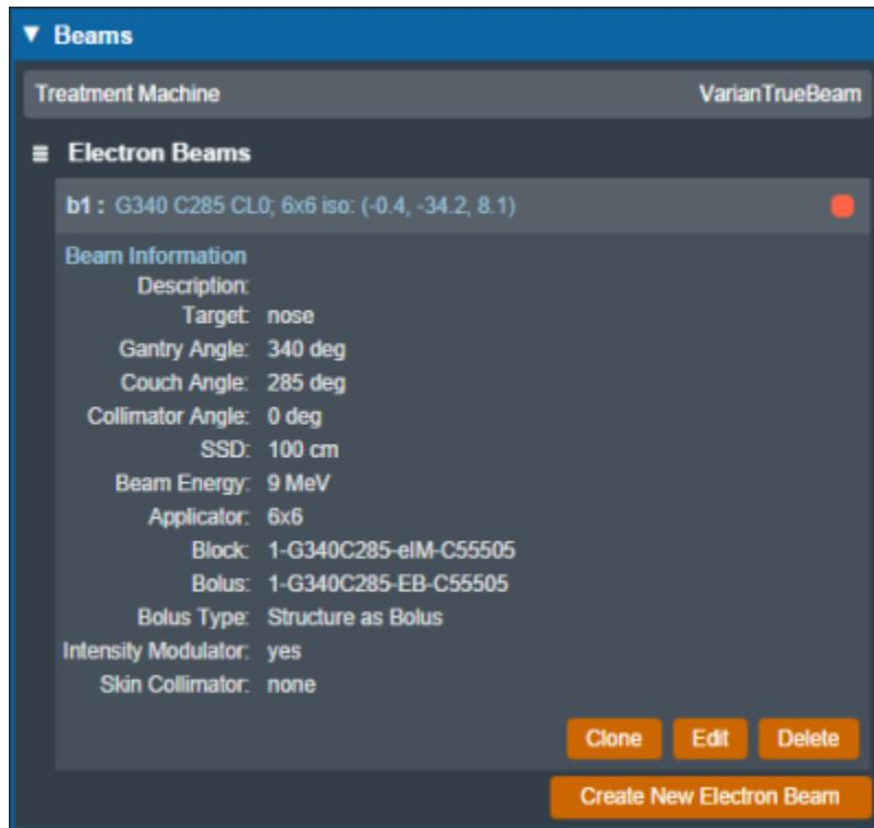
Fig. 2: Existing Beam Example
