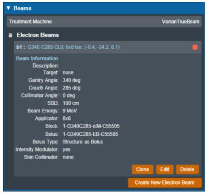
Fig. 2: Existing Beam Example
