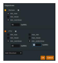
Once all the *Objectives* have been set, the user is ready to run the MCO solver, which is performed in the *Objectives/Optimizer* block.
