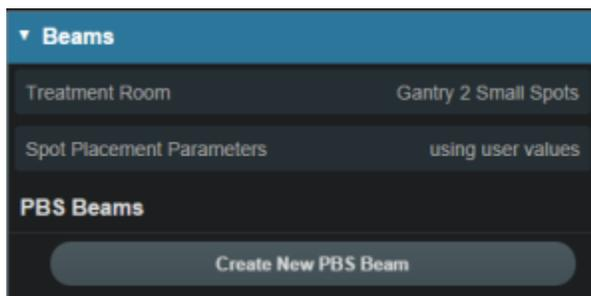
5. After you select the *Create New PBS Beam* you will be able to set the beam geometry parameters:
