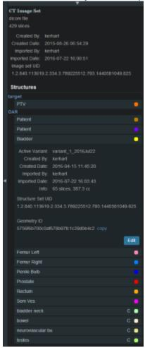
4. Structures not defined in the site config (a custom structure) are denoted with a "c" beside it. These structures have the ability to be edited in a limited capacity. The planner may choose to change the structure variant, color, and structure type. The planner may also choose to enter any notes that may be helpful at this point.
