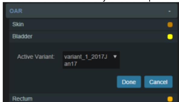
4. Structures not defined in the site config (i.e. custom structures) are denoted with a “c” beside it. These structures have the ability to be edited in a limited capacity. The planner may choose to change the structure variant, color, and structure type. The planner may also choose to enter any notes that may be helpful at this point.
